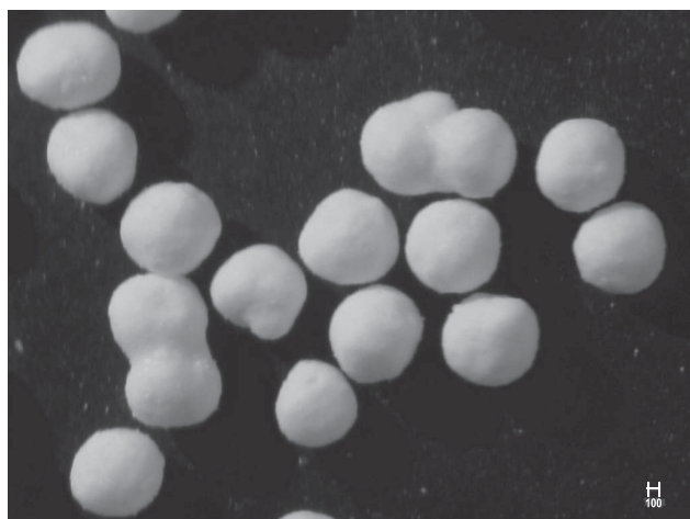
FIGURE 3. Pellets containing the sucrose starters as observed under the optical microscope. The measure bar corresponds to 100 \mu\text{m} .
